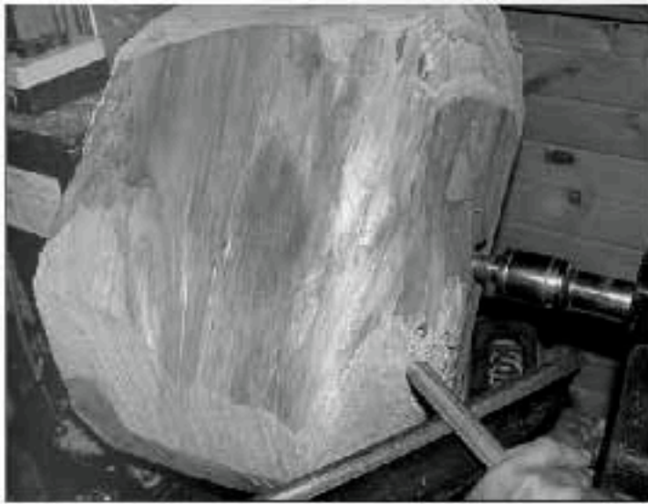
Now we are into a red zone: large diameter (17"), heavy, out-of-round/balance blank. If the lathe can handle such a piece, I progress from a point just below vibration to a modest speed as it becomes more balanced. However, with a rim speed of 51mph at 1,000 rpm, I never find it necessary to crank up much speed.
