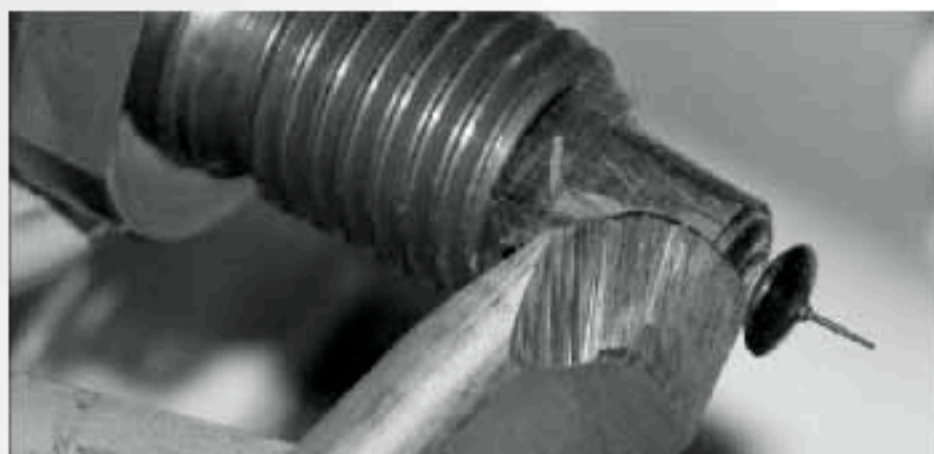
When working small diameter miniatures, you really can raise the speed to fairly high levels. However, I was getting clean cuts on this \frac{3}{8} " piece at speeds easily below 1,000 rpm.
